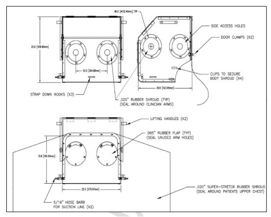
Figure 2 Sketch indicating location of six exterior arm shrouds and plates, six interior arm shrouds and plates, one interior flap and body shroud, suction valves and barbs.
