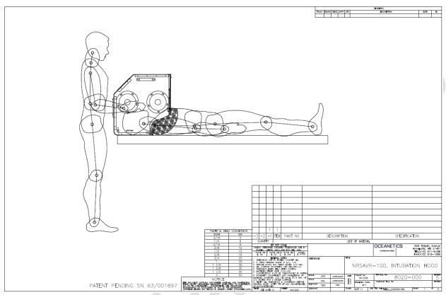
Figure 1 NRSAVR-100 General Assembly Drawing Number 8020-000.
